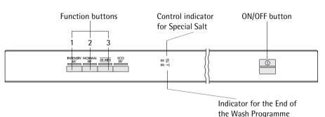
**Function buttons:** In addition to the dishwashing cycle the following functions can also be set with the help of these buttons:
